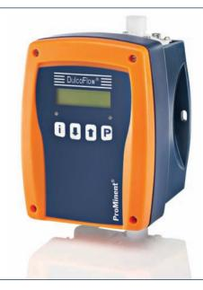
The flow meter DulcoFlow® measures all liquid media by detecting the flow volume of pulsing liquids. The instrument is based on the ultrasonic measurement method. Parts that come into contact with the media are manufactured from chemically resistant PVDF/PTFE. This ensures that aggressive media can also be measured without problem. The instrument is installed directly in the pipe of the medium being measured.
